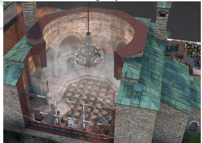
Figure 13: Thermal heating system- behind the walls (Mozaik Education, 2023)
