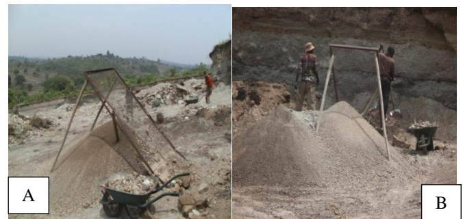
Figure 6: Plate showing Materials used for sand extraction in Baleng
