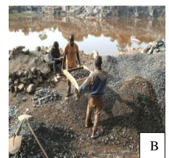
Figure 12: Plate showing gravel exposure and gravel screening
