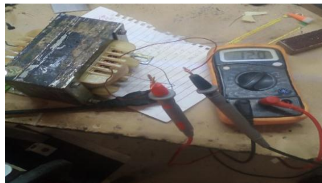
Figure 8: Designed sample transformer showing output voltage (12.0VAC)
