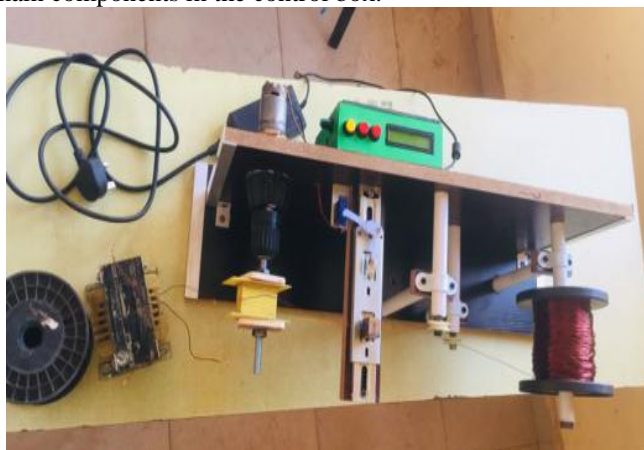
Figure 7: Assembled transformer winding machine and accessories
