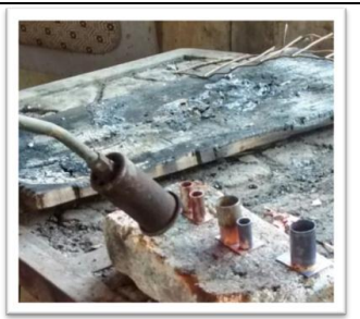
Plate 12: Soldering the cylinders
