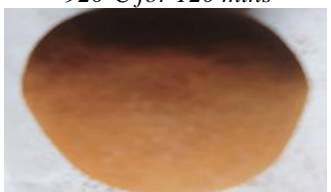
Figure 18a: Pellet Itakpe @ 960^{\circ}\text{C} for 120 mins
