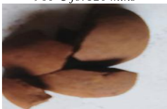
Figure 19 a: Pellet Itakpe @ 1000^{\circ}\text{C} for 120 mins
