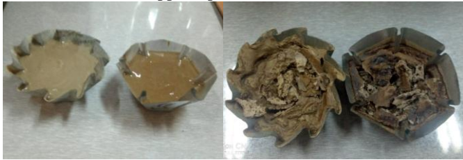
Figure 2: Mud Samples showing ENV and INV Mud: before Drying (Left) and after Drying (Right)
