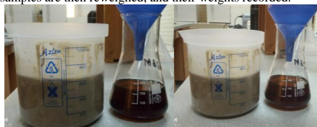
Figure 1: Centrifuged Samples showing Liquid and Semi-Solid Phases of ENV (Left) and INV (Right)
