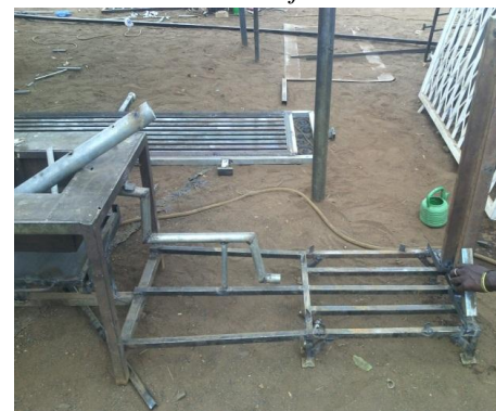
Plate 40: Finished joined burner frame with bellow stand FINISHING: was the last and final process of which the researchers used grinder to grind certain rough areas, filled some areas with filler and sanded it to make it levelled and smooth for spraying.
