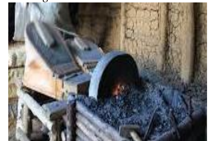
Figure 8: Metal and clay made burner
