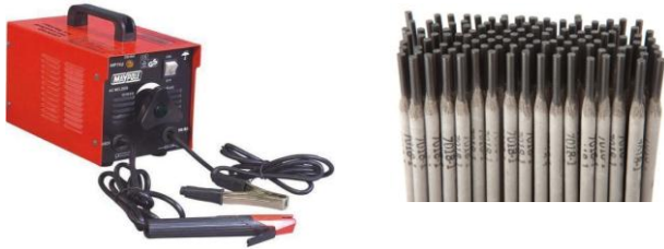
Plate 17: Welding machine and electrode were used in the joining process
