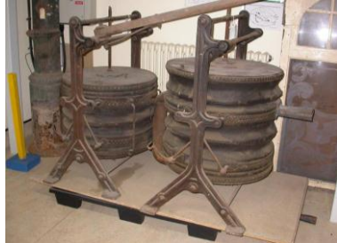
Figure 2: Hand operated bellow
