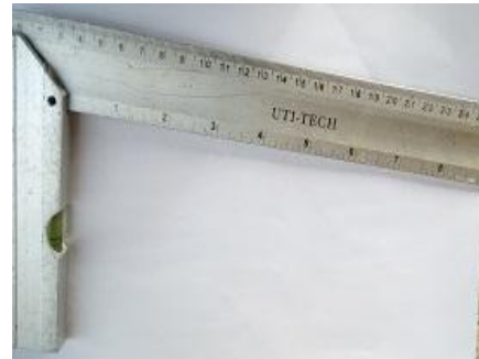
Plate 13: 90° angle ruler was used in checking straightness of the work at its angles
