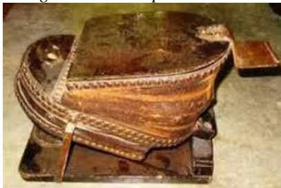
Figure 3: Hand operated bellow
