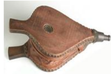
Plate 3: A hand operated bellow in metal, wood and leather
