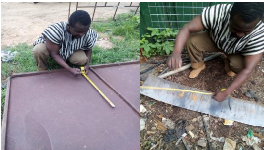
Plate 36: Taking measurement of the galvanised sheet to form the burner by the researchers
