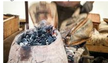
Figure 9: Clay-fibre made burner
