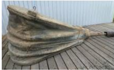
Figure 1: Hand operated bellow
