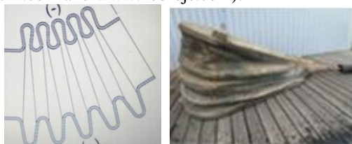
Figure 12: Angular Types of Bellow
