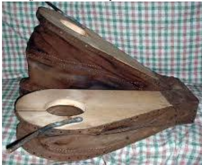
Figure 4: Leg operated bellow
