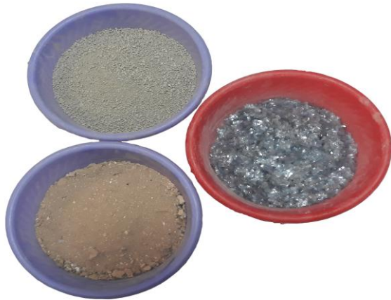
Figure 1: Natural Soil, Brick Kiln Dust and Plastic Bottle Strip
