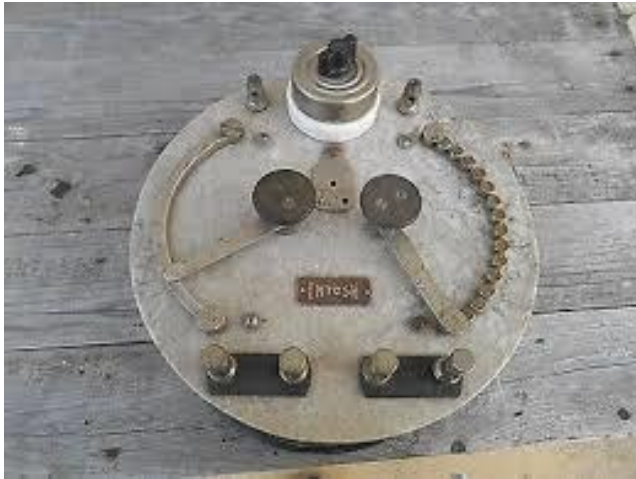
Old electrical dimmer
