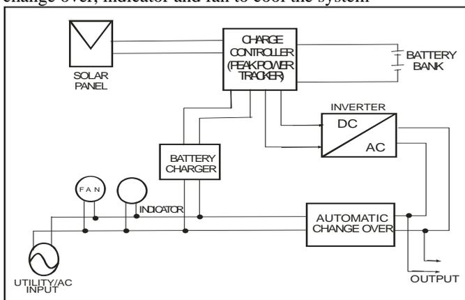
Figure 1: Block Diagram of the Circuit
