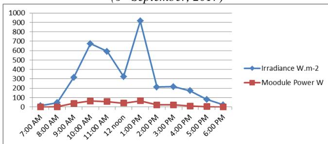
Figure 3: Comparison of Available Solar Irradiance and Module Power (6th September, 2017)
