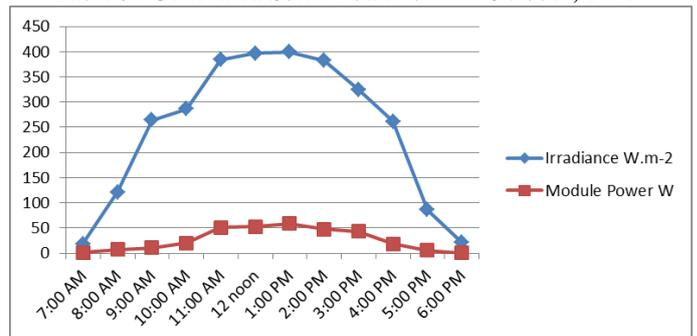
Figure 6: Comparison of Available Solar Irradiance and Module Power (6th October, 2017)
