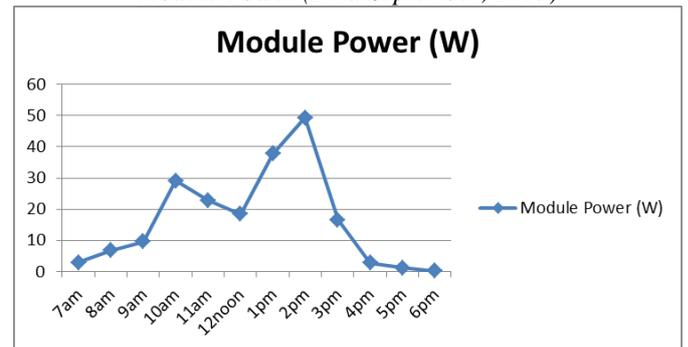
Figure 5: Graph of Module Power Against Time of the Day (23rd September, 2017)
