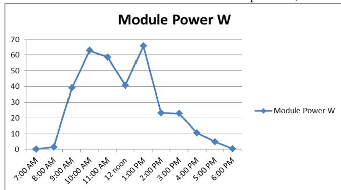
Figure 2: Graph of Module Power Against Time of the Day (6<sup>th</sup> September, 2017)
