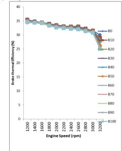
Figure 4: Variation of Brake Thermal Efficiency with Engine Speed At 80% Load
