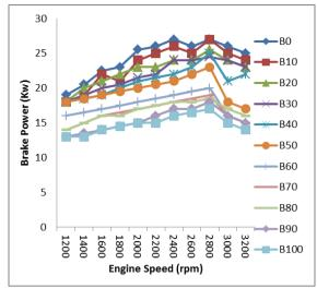
Figure 2: Variation Of Brake Power With Engine Speed At 80% Load
