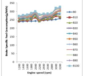
Figure 3: Variation of Brake Specific Fuel Consumption with Engine Speed At 80% Load
