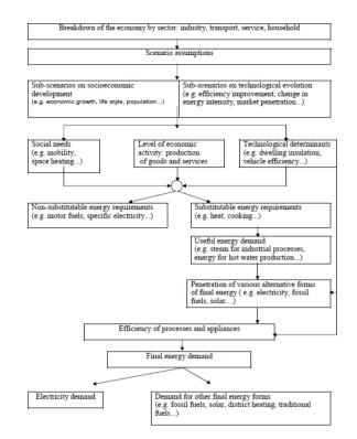
Source: IAEA MEAD model manual 2008 Figure 2: Scheme used to project useful and final energy demand in MAED
