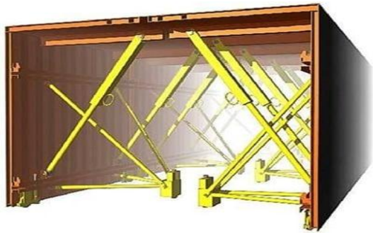
Figure 2: Tunnel form work for wall and slab
