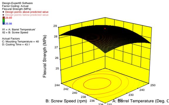
Figure 2: graph of screw speed and barrel temperature effect on flexural strength
