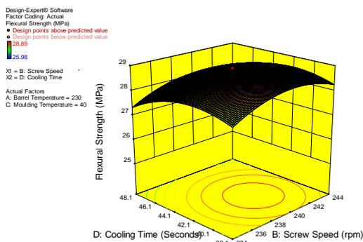
Figure 5: graph of cooling time and screw speed effect on flexural strength
