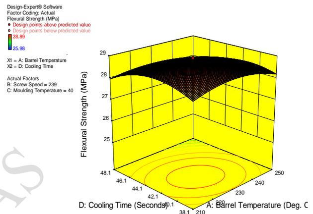
Figure 7: flexural strength – Cooling time and barrel temperature curve
