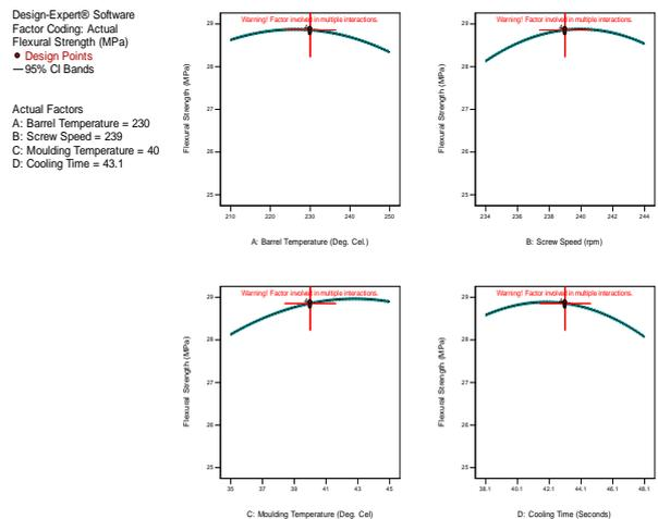
Figure 8: flexural strength – All factors curve
