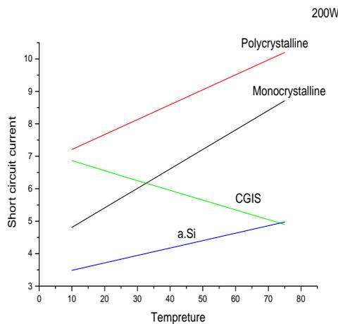
Figure 4: Variation of Short circuit current with temperature at fixed irradiance ( $1000W/m^2$ ) for the three PV module technologies rated at 220W and 200W
