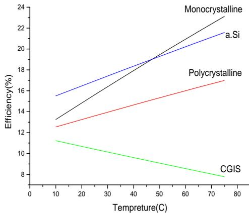
Figure 3: Variation of efficiency with temperature at fixed irradiance ( $1000W/m^2$ ) for three the PV module technologies rated at 220W and 200W
