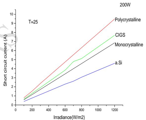
Figure 5: Variation of Short circuit current with irradiance at fixed Temperature ( $25^{\circ}C$ ) for the three PV module technologies rated at 220W and 200W
