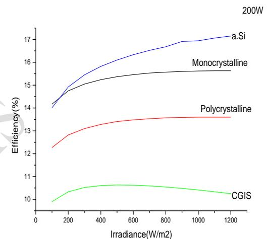
Figure 2: Variation of efficiency with irradiance at fixed Temperature (25°C) for the three PV module technologies rated at 220W and 200W
