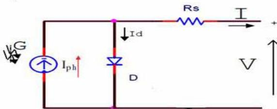
Figure 1: A one diode equivalent circuit PV Cell
