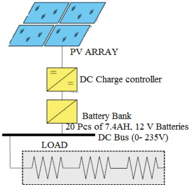
Figure 2: Developed System.
