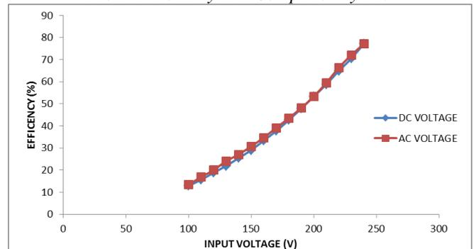
Figure 3: Efficiency Characteristic of Resistive load
