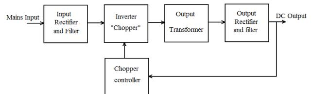
Figure 1: Block Diagram of Switch Mode Power Supplies
