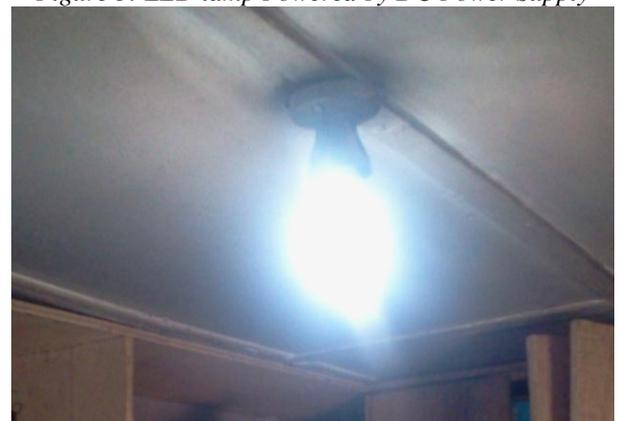
Figure 6: CFL lamp Powered by DC Power Supply
