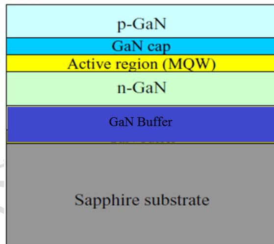
Figure 2: Structure of the fabricated white LED
