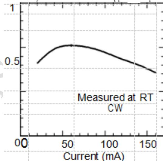
Figure 5: External quantum Efficiency of a quarternary InAlGa<sub>N</sub> based UV-LED fabricated on a GaN/sapphire template
