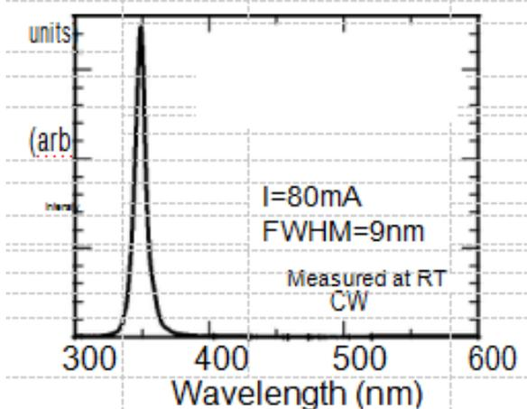
Figure 3: Electroluminescence (EL) spectrum of a quarternary InGa<sub>N</sub> based UV-LED fabricated on a GaN/sapphire template
