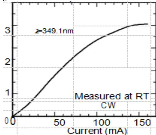
Figure 4: I-L characteristics of a quarternary InAlGa<sub>N</sub> based UV-LED fabricated on a GaN/sapphire template
