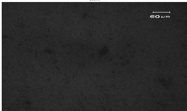
Figure 8: OM micrograph for Al6061 + 2.5% Red mud
