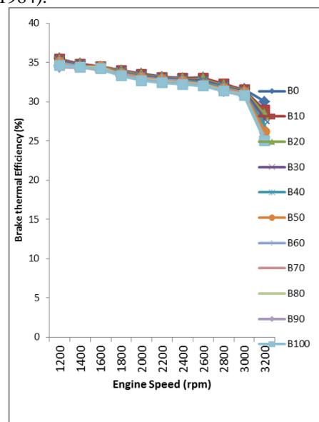
Figure 4: Variation of Brake Thermal Efficiency with Engine Speed At 80% Load
