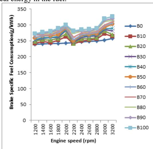
Figure 3: Variation of Brake Specific Fuel Consumption with Engine Speed At 80% Load
