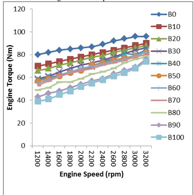
Figure 1: Variation of Engine Torque with Engine Speed At 80% Load
