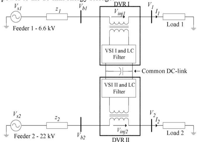
Figure 2: A simplistic IDVR system with two DVRs connected to dc link
