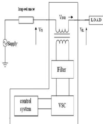
Figure 1: Schematic diagram of DVR
