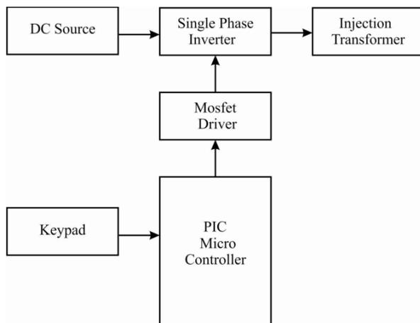
Figure 4: Block Diagram of Proposed Hardware Model
