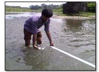
Plate 9.4: Velocity measurement during field Survey
