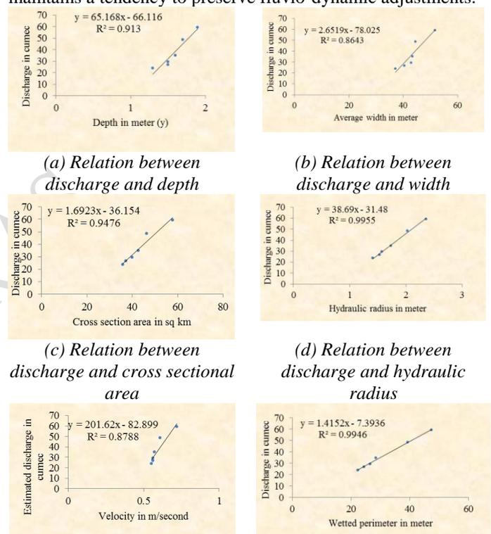
Figure 7.1: Interrelationship between hydraulic parameters (no. a-d)
