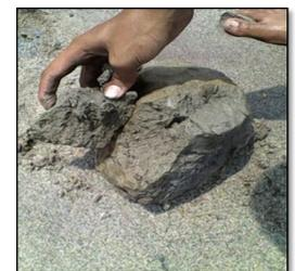
Plate 9.6: Clayey bed material offering low frictional and moderate Resistance energy
