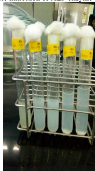
Figure 1: Alkaline phosphatase Enzyme Inhibition by mercuric chloride resulting in to no color change
