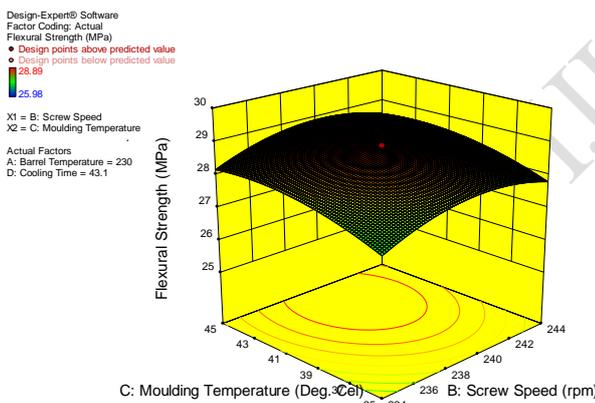
Figure 4: graph of moulding temperature and screw speed against flexural strength
