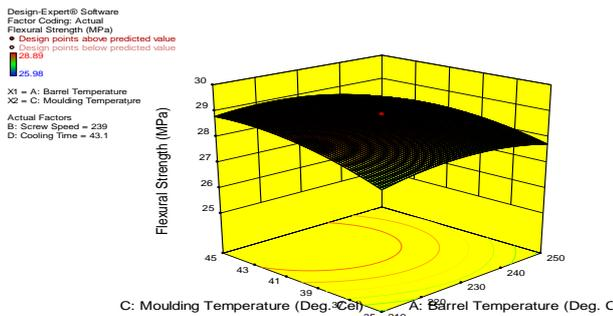
Figure 3: graph of flexural strength effect against moulding temperature and barrel temperature
