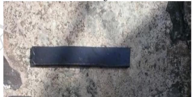
Figure 1: Flexural Strength Test Specimen
