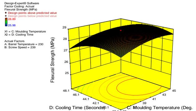
Figure 6: graph of flexural strength against cooling time and moulding temperature
