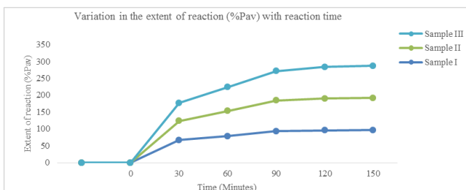
Figure 2: variation in extent of reaction (%P av ) with time
