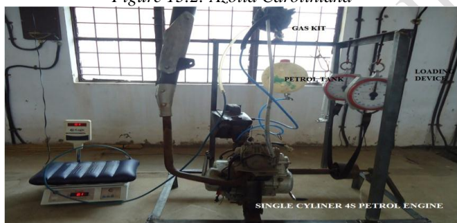
Figure 13.3: Load test bed assembly
