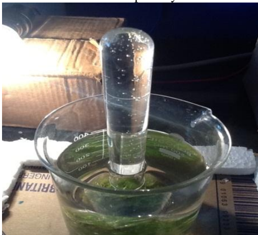
Figure 15: Air bubbles accumulated on the top of test tube, which was covered with blue colour filter
