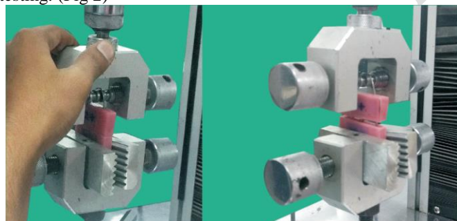
Figure 2: Retention force Measurement Using Universal Testing Machine
