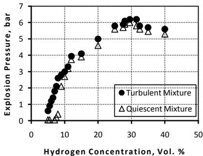
Figure 8: Effect of turbulence on maximum explosion pressure for hydrogen-air mixture (ignition at centre of sphere)
