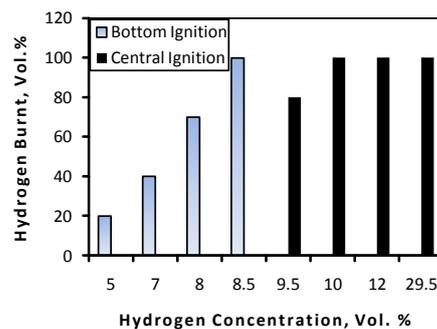
Figure 6: Hydrogen burnt as a function of initial hydrogen concentration in hydrogen-air mixture
