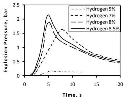
Figure 2: Explosion pressure curves for hydrogen-air-mixtures (ignition at 0.30 m from the bottom of sphere)
