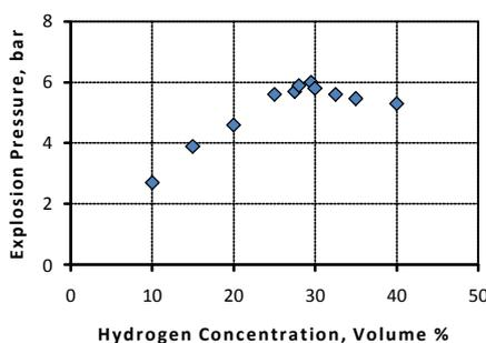
Figure 5: Variation of maximum explosion pressure with hydrogen concentration
