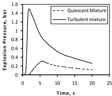
Figure 7: Effect of turbulence on explosion of hydrogen-air mixture (6% hydrogen in air, ignition at 0.30 m from bottom of sphere)
