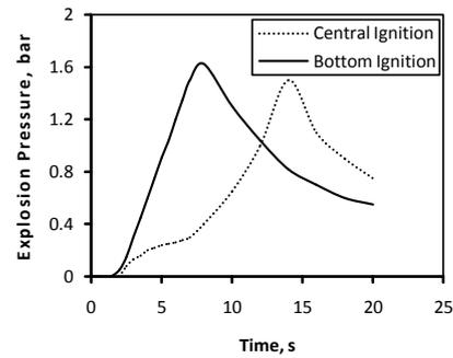
Figure 9: Effect of location of ignition source on maximum explosion pressure for hydrogen-air mixture (7% hydrogen in air)
