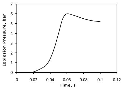
Figure 4: Explosion pressure-time history for stoichiometric hydrogen-air mixture
