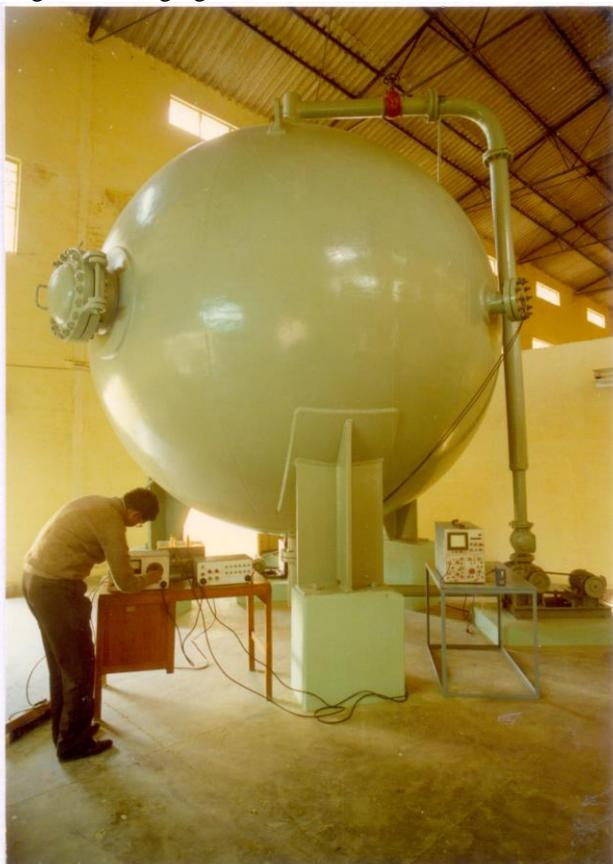
Fig.1. Large- 3.66-m diameter Spherical Vessel for explosion research studies
