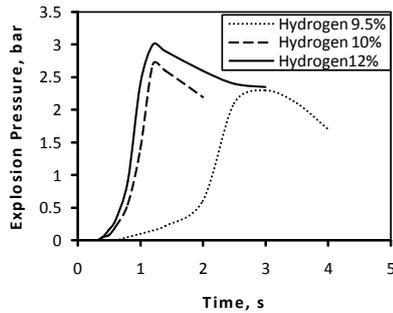
Figure 3: Explosion pressure curves for hydrogen-air mixtures (ignition at centre of sphere)
