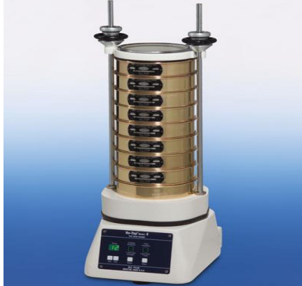
Figure 4: Segregating the filler using sieve shaker
