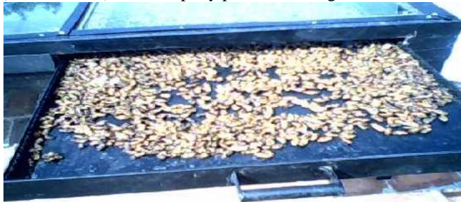
Figure 8: A tray with solar absorber (aluminum sheet)
