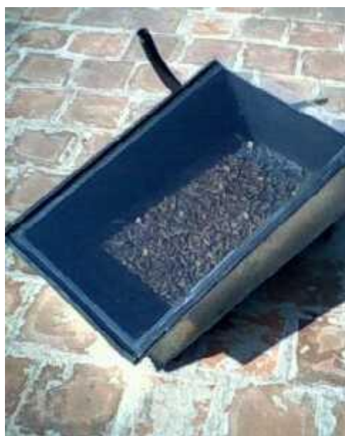
Figure 5: Solar Pupae Drier (SPD) with glass pane and chimney
