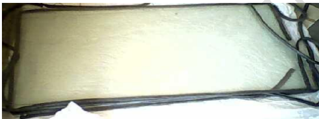
Figure 9: Toughened solar glass with rubber beadings
