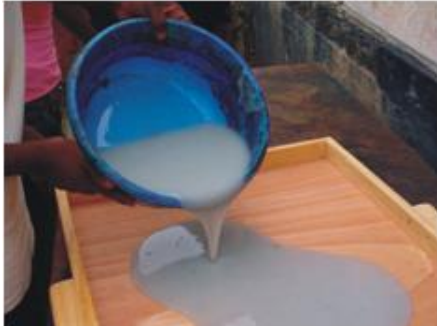
Plate 3: Pouring starch into trough
