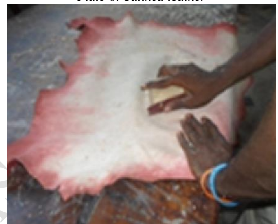
Plate 9: Sanding on flesh side of leather
