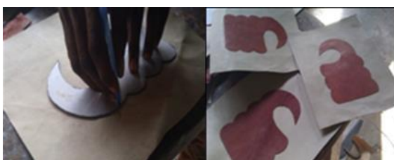
Plate 16: (Marking of Akoben template and pasting on leather)
