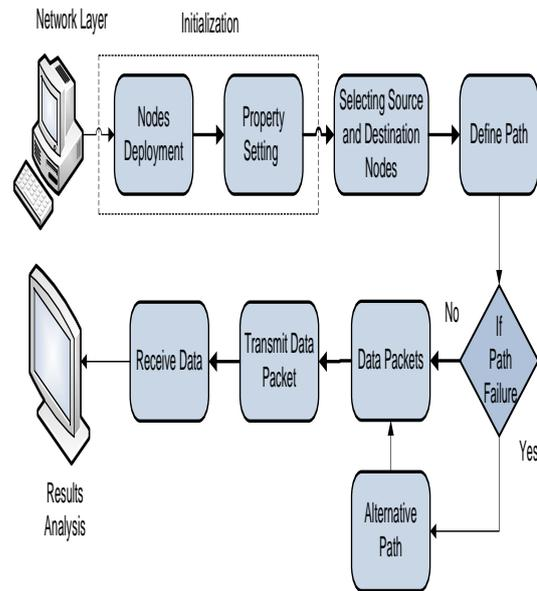
Figure 1: proposed architecture of path selection
