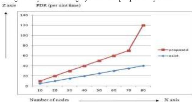
Figure 8: Comparison Graph for Packet Delivery Ratio
