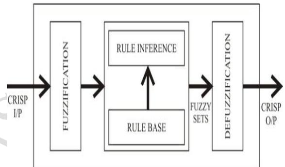
Figure 2: Schematic of fuzzy logic control
