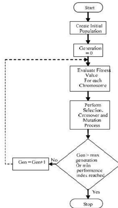
Figure 4: Implementation of Genetic Algorithm based controller
