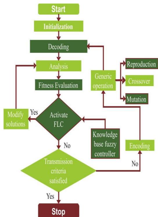
Figure 5: Block diagram of hybrid fuzzy logic genetic algorithm
