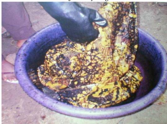
Figure 5: The waxed printed fabric being dyed
