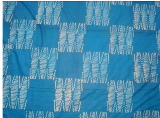
Figure 14: Waxed printed fabric ready to be dyed yellow
