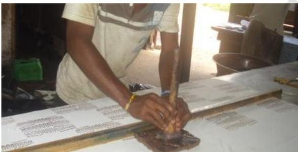
Figure 11: Waxing fabric with a wooden designed block
