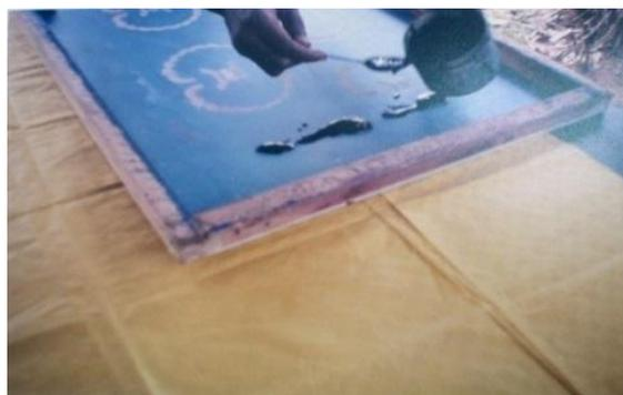
Figure 2: Pouring the print paste unto the screen for printing
